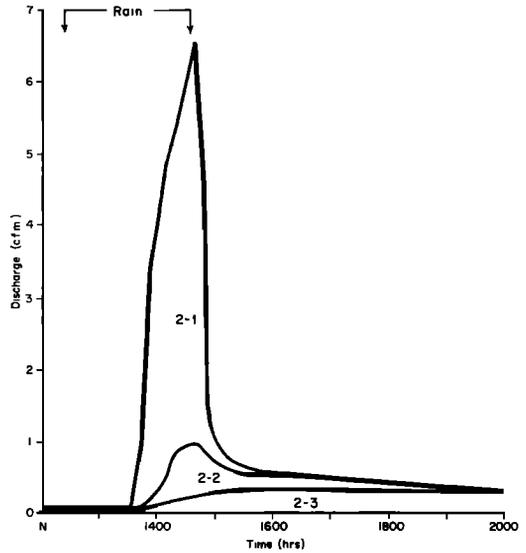
Fig. 6. Combined hydrograph of flows from plot 2 (concave) during the artificial storm of October 25, 1967.
