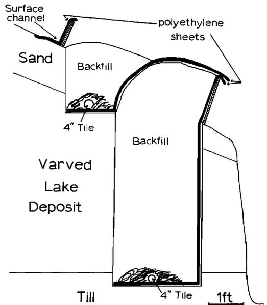
Fig. 3. Cross section of the interceptor trench.
