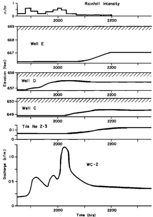
Fig. 4. Rainfall, changes in water-table elevation, and runoff from tile 2-3 and weir WC-2 during and after the 0.70-inch rainstorm of October 18, 1967.
