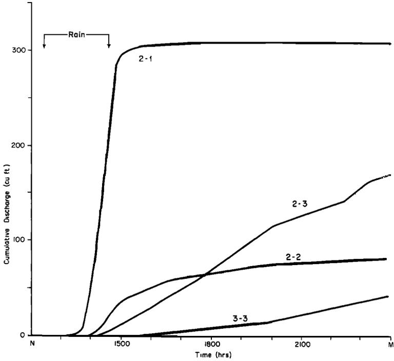
Fig. 7. Cumulative flow for the tiles producing runoff during and after the storm of October 25, 1967.
