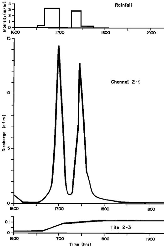
Fig. 10. Rainfall and runoff data for plot 2 (concave) in the natural storm of July 17, 1968.
