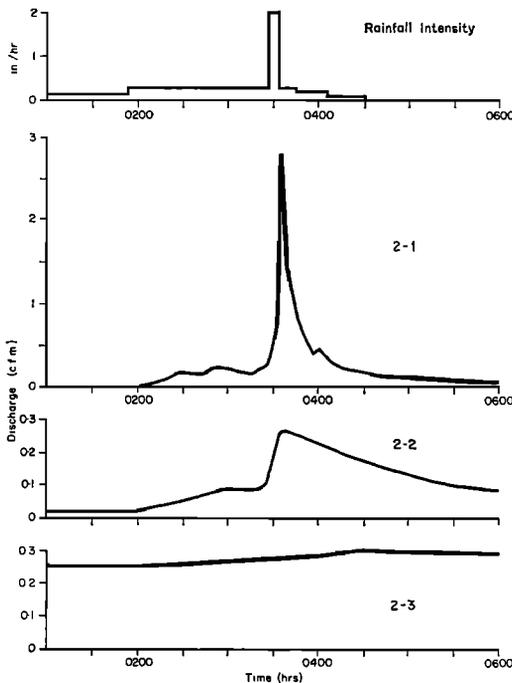
Fig. 9. Rainfall and runoff data from plot 2 for the 0.88-inch natural storm of October 26, 1967.
