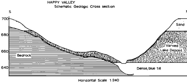
Fig. 2. Schematic geological cross section of the experimental area.
