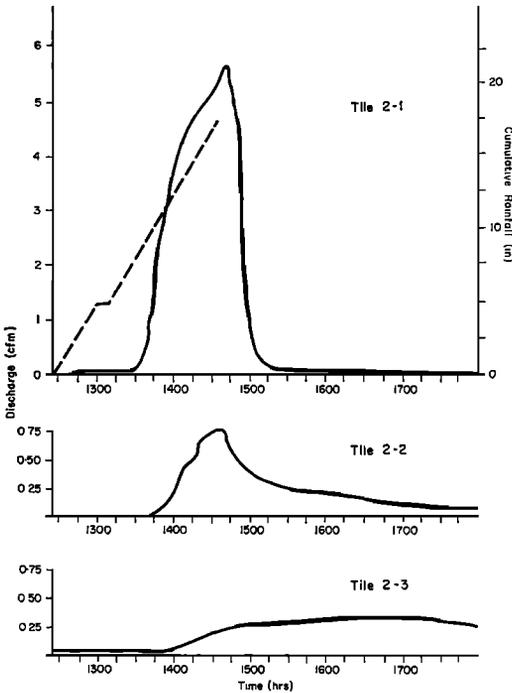
Fig. 5. Discharge from the three tiles draining plot 2 (concave) during and after the artificial storm of October 25, 1967.
