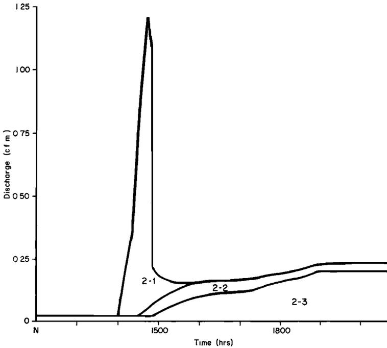
Fig. 8. Combined hydrograph of runoff from plot 2 during the storm of October 16, 1967.
