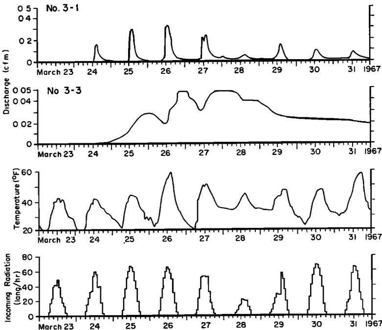
Fig. 5. Air temperature, incoming shortwave radiation, and runoff from plot 3 during the snowmelt period of March 1967.
