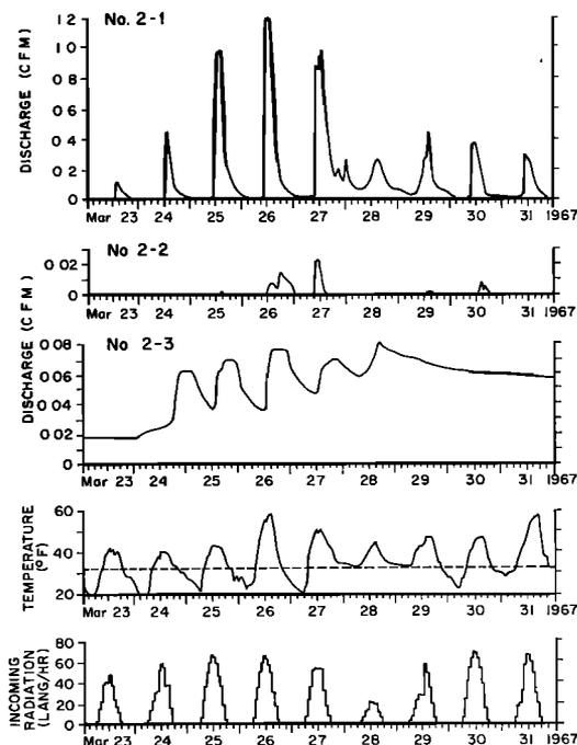
Fig. 3. Air temperature, incoming shortwave radiation, and runoff from plot 2 (concave) during the snowmelt period of March 1967.
