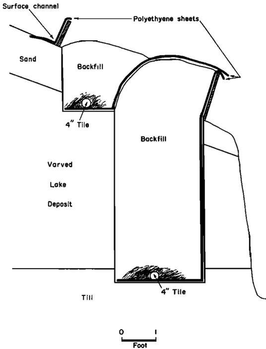
Fig. 2. Cross section of the interceptor trench.
