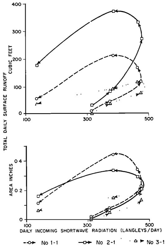
Fig. 8. Relationship between daily totals of incoming shortwave radiation and surface runoff for the three plots on the trenched hillside during the snowmelt period of March 1967.
