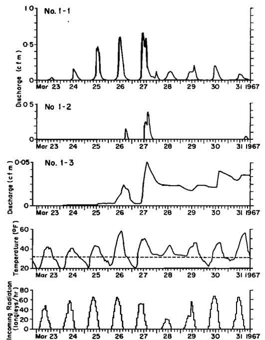
Fig. 4. Air temperature, incoming shortwave radiation, and runoff from plot 1 during the snowmelt period of March 1967.
