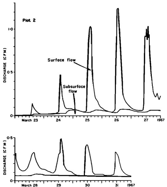
Fig. 9. Combined hydrograph of surface and subsurface flow from plot 2 (concave) during the snowmelt period of March 1967.
