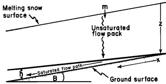
Fig. 1. The path of water flow through the snowpack.
