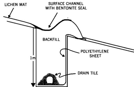
Fig. 2. The runoff collection system.
