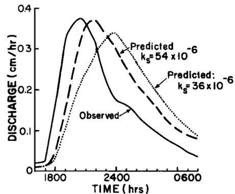
Fig. 7. Observed hydrograph and calculated outflow from the saturated layer at the base of plot A on the tundra, May 16, 1972. Two outflow hydrographs were computed by using different values for  $k_s$  with  $k_u$  held constant at  $6 \times 10^{-6} \text{ cm}^2$ .
