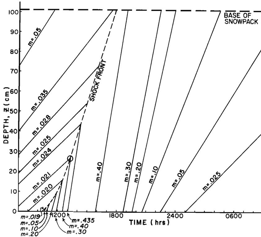
Fig. 6. Speed of values of constant flux rate originating at the surface of the snowpack ( $z = 0$ ) at various times as indicated on Figure 5. The times at which these flux rates intersect the base of the snowpack determines the hydrograph of the input to the saturated layer.
