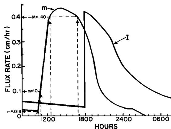
Fig. 5. Computed rates of surface melting  $m$  and output from the unsaturated zone into the saturated layer  $I$  for plot A on the tundra, May 16, 1972. Snow depth was 101 cm.
