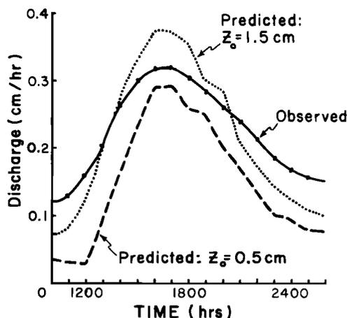
Fig. 10. Effect on the predicted hydrograph of changing the roughness length ( $z_0$ ) of the snow surface on a day with high turbulent heat flow to the snowpack of plot G in the forest on May 11, 1973. Daily total melt calculated with  $z_0 = 0.5$  cm was 3.11 cm; with  $z_0 = 1.5$  cm, the calculated melt was 4.18 cm; the observed melt was 4.95 cm.
