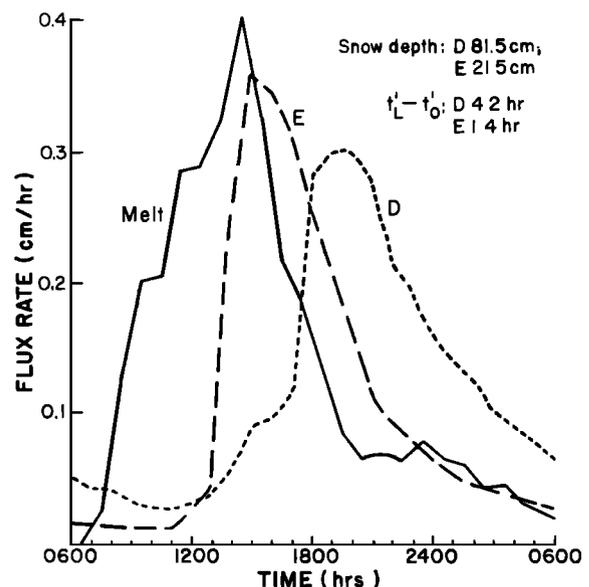
Fig. 3. Hydrographs of surface melting and runoff from plots D and E in the boreal forest on May 9, 1973.
