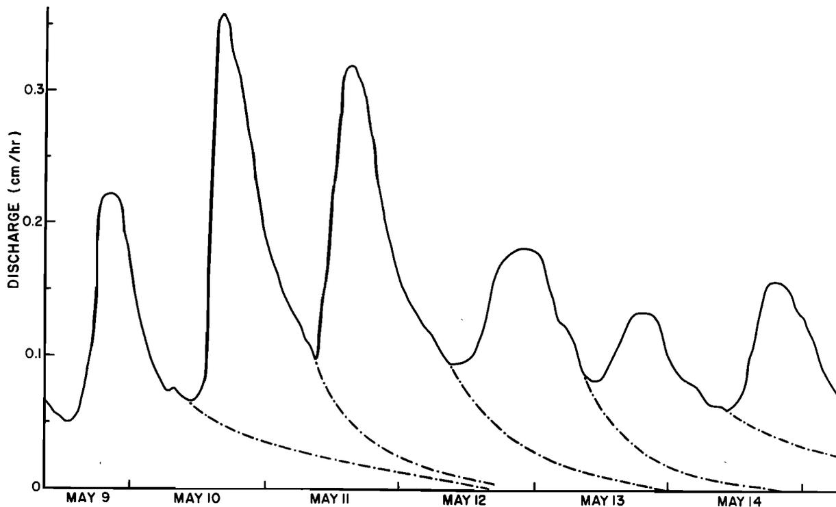
Fig. 4. Hydrographs of surface runoff from plot G in the forest in May 1973.
