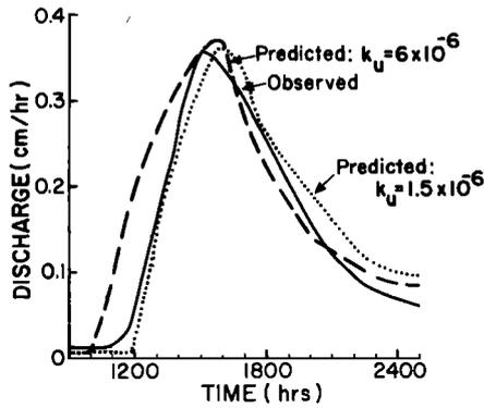
Fig. 8. Observed hydrograph and calculated outflow from the saturated layer at the base of plot E in the forest, May 9, 1973. Two outflow hydrographs were computed by using different values for  $k_u$  with  $k_s$  held constant at  $54 \times 10^{-8} \text{ cm}^2$ .
