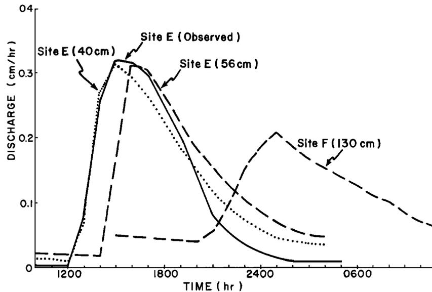
Fig. 9. Observed hydrograph and hillslope discharge from plot E computed by using the actual snow depth of 56 cm and a hypothetical snow depth of 42 cm. The computed outflow hydrograph from plot F is also shown. Because of instrument failure the hydrograph from plot F was not measured, but the predicted and observed hydrographs from this plot agreed closely on other days.
