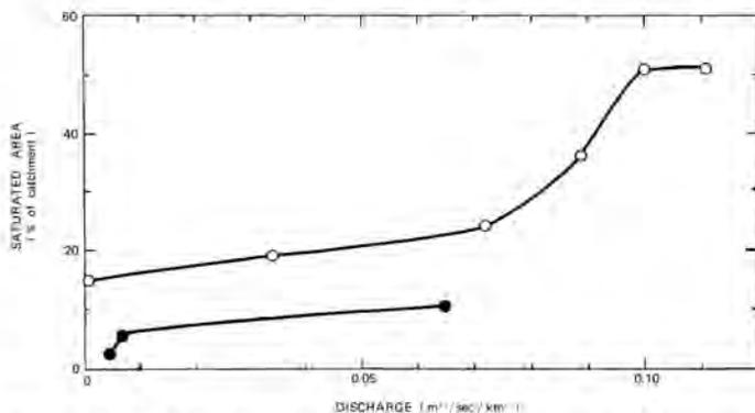
Figure 4. Relation between baseflow and the extent of the saturated area in two Vermont catchments.
