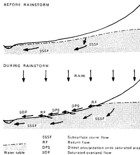
Figure 1. Runoff-producing processes in a humid-region catchment during a rainstorm.
