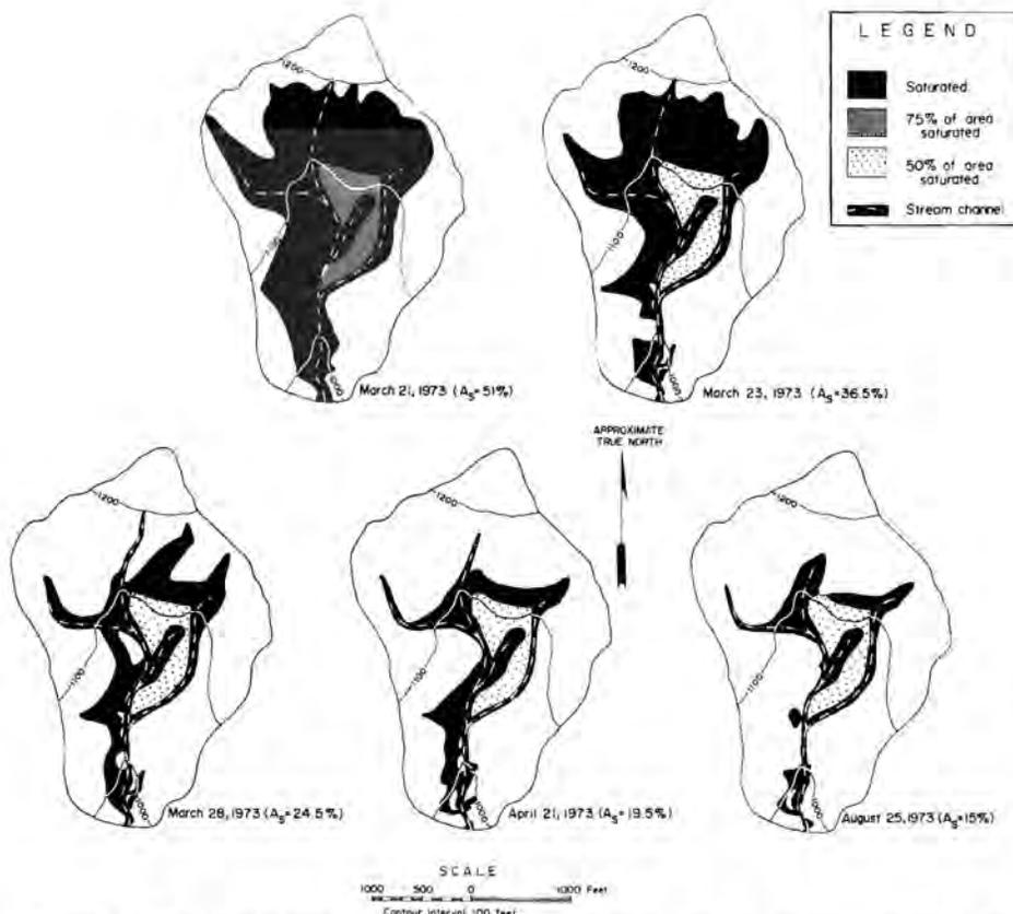
Figure 2. Seasonal extent of the saturated area before summer storms, autumn storms, and immediately after snowmelt in a Vermont catchment with steep, well-drained slopes and a narrow valley bottom.
