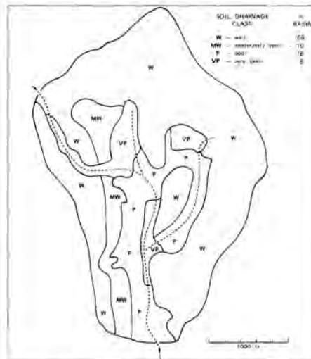
Figure 3. Soil drainage class map of the Vermont catchment (Figure 2).
