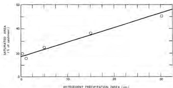
Figure 5. Relation between antecedent precipitation index and the extent of the saturated area in the Vermont catchment (Figure 2).
