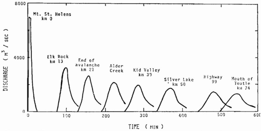
**Figure 5 :** Hydrographs of mudflows originating from a pyroclastic flow onto a snowpack and routed downvalley to the mouth of the Toutle valley. This computation involved routing through 243 segments, 300 m in length.
