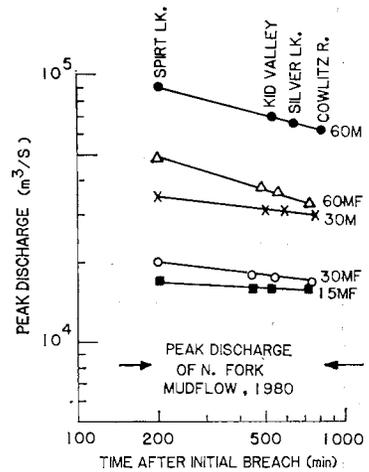
**Figure 8 :** Computed peak discharges of mudflows and muddy floods generated under various hypothetical scenarios for the potential breaching of the Spirit Lake debris barrier. The number on each curve indicates the maximum depth of incision of the barrier allowed in the calculation of the initial outburst hydrograph. The letters M and MF refer to a mudflow and a muddy flood respectively.
