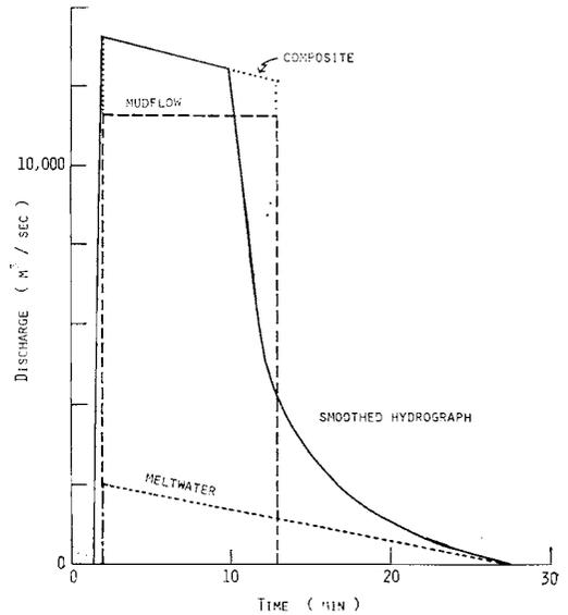
**Figure 3:** Hydrograph of a mudflow combined with a snowmelt flood to yield a composite hydrograph, which was smoothed slightly to reflect progressive failure of the mudflow material and variations of velocity and ponding along the mudflow track, and to facilitate routing calculations.
