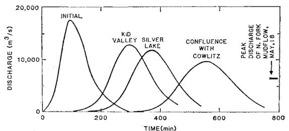
Figure 7: Computed hydrographs of a muddy flood generated by the potential breaching of the Coldwater debris barrier, releasing water at a peak rate of 18,000 m<sup>3</sup>/s. The hydrographs were routed downstream by the Muskingum procedure.
