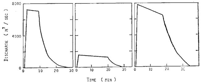
**Figure 4:** Examples of mudflow hydrographs computed from alternative assumptions concerning the contributions of meltwater runoff and mudflow discharges resulting from a pyroclastic flow over snow. The peak discharges differ under these assumptions but each scenario shows a decline in discharge to small values within 30 minutes.
