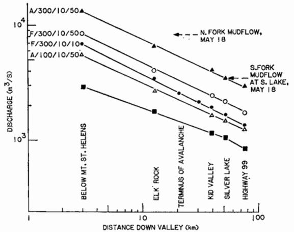
**Figure 6 :** Downstream variation of peak discharge for mudflows originating from pyroclastic flows and routed downvalley. Assumed conditions governing the initial hydrograph are summarized by labels at the upper left. The sequence of symbols in these labels refer to scenarios in Table 2, as follows: month of average snowpack used; width of mudflow track; speed of mudflow; depth of snowmelt on fan. Also shown are field estimates of peak discharges for the mudflows of May 18, 1980.
