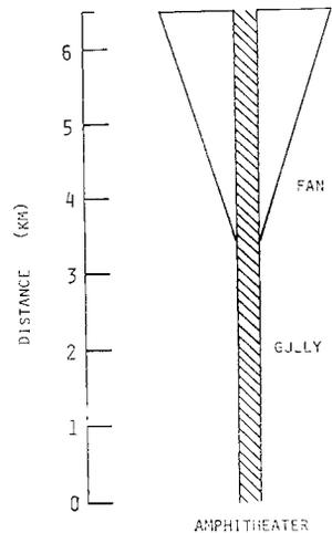
**Figure 2 :** Schematic representation of the area over which a pyroclastic flow would travel north from the crater of Mt. St. Helens. In the worst case, all snow would be eroded and melted in the steep, narrow upper part of the track, and the resulting mudflow would erode the snow in a track indicated by the cross-hatched area. The pyroclastic flow would spread from the gully to the triangular area indicated at a distance of 3.5–6.5 km from the center of the crater.
