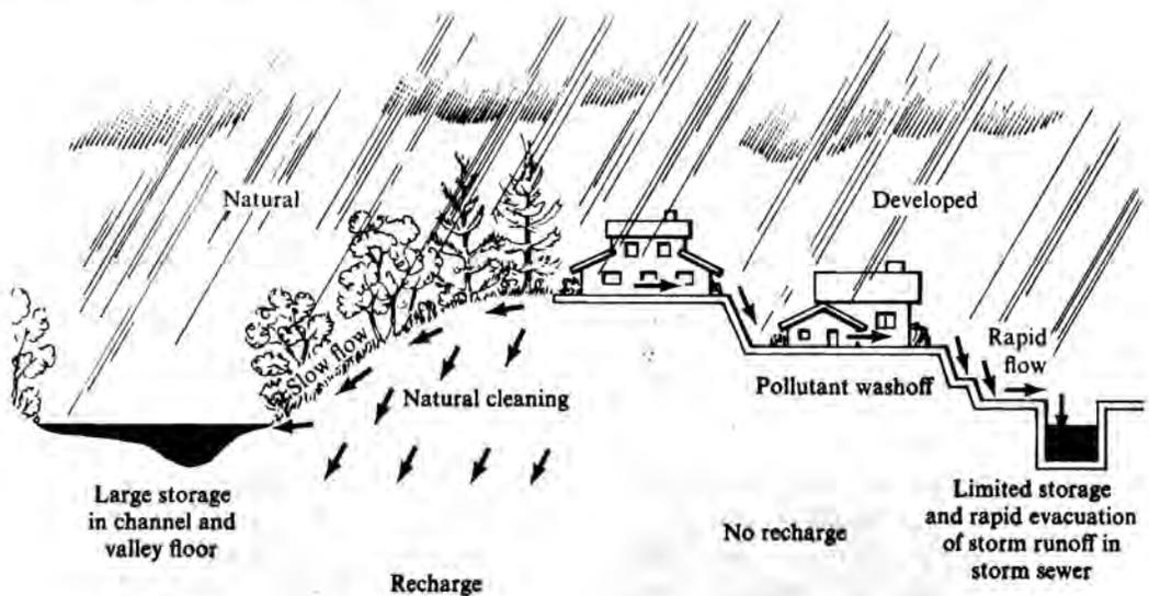
Figure 1. Schematic representation of the problems to be managed in the control of urban storm runoff. (Source: Dunne and Leopold, *Water in Environmental Planning*, Copyright W.H. Freeman Co., 1978).
