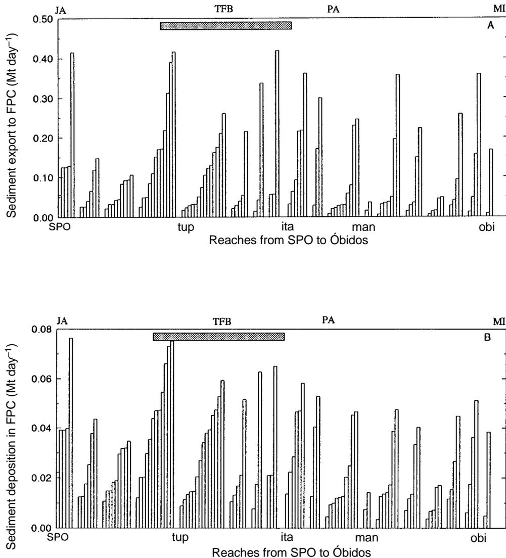
**Figure 8.** Computed daily rates of (A) sediment export into and (B) deposition within each of the 105 flood-plain channels at peak flow. Note the difference in ordinate scales. The bars indicate each value within a sampling reach and do not imply downstream increases within each reach. Abbreviations as in Figure 3.
