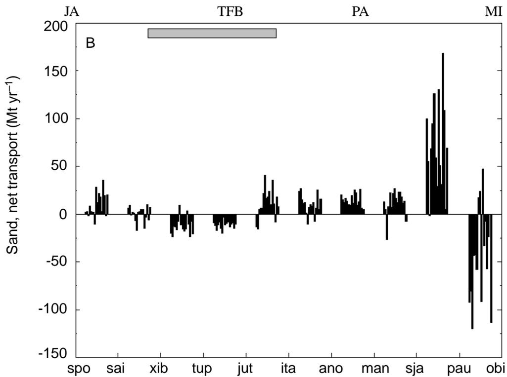
Figure 5. Net suspended sediment transport for each reach and for each year 1974–1989. (A) Silt-clay. (B) Sand. Positive values indicate that more sediment was transported into the channel reach than out of it, and therefore was accumulated within the reach. Note the difference in ordinate scales. Abbreviations as in Figure 3.
