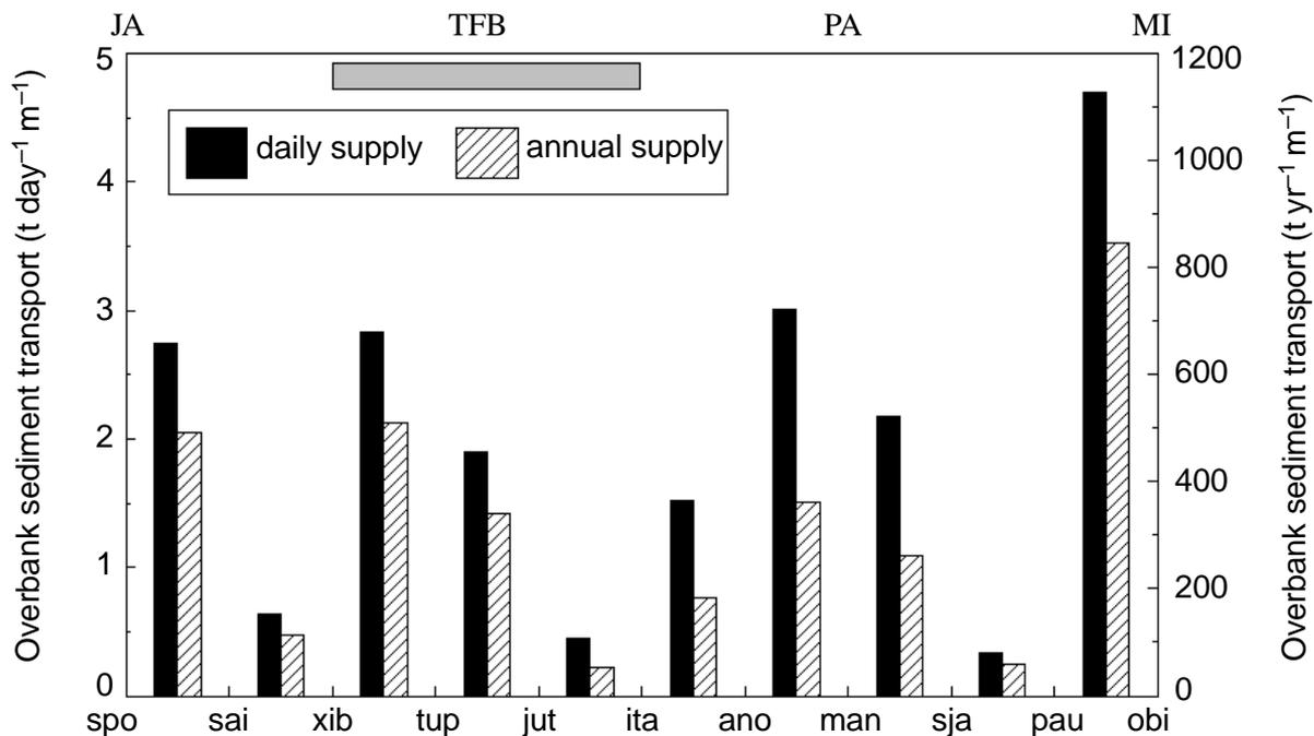
**Figure 7.** Computed rates of sediment transport in diffuse overbank flow. The left bar of each pair indicates the average daily rate of transport per meter over each bank during the season of overbank flow, calculated from flood routing of daily flows throughout 1974–1989. The right bar of each pair indicates the average annual overbank transport per meter. Abbreviations as in Figure 3.
