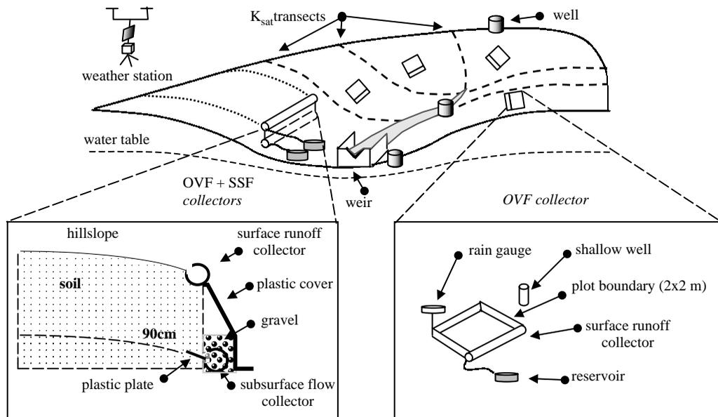
Figure 4. Schematic of the field measurements in the pasture and the forest catchments
