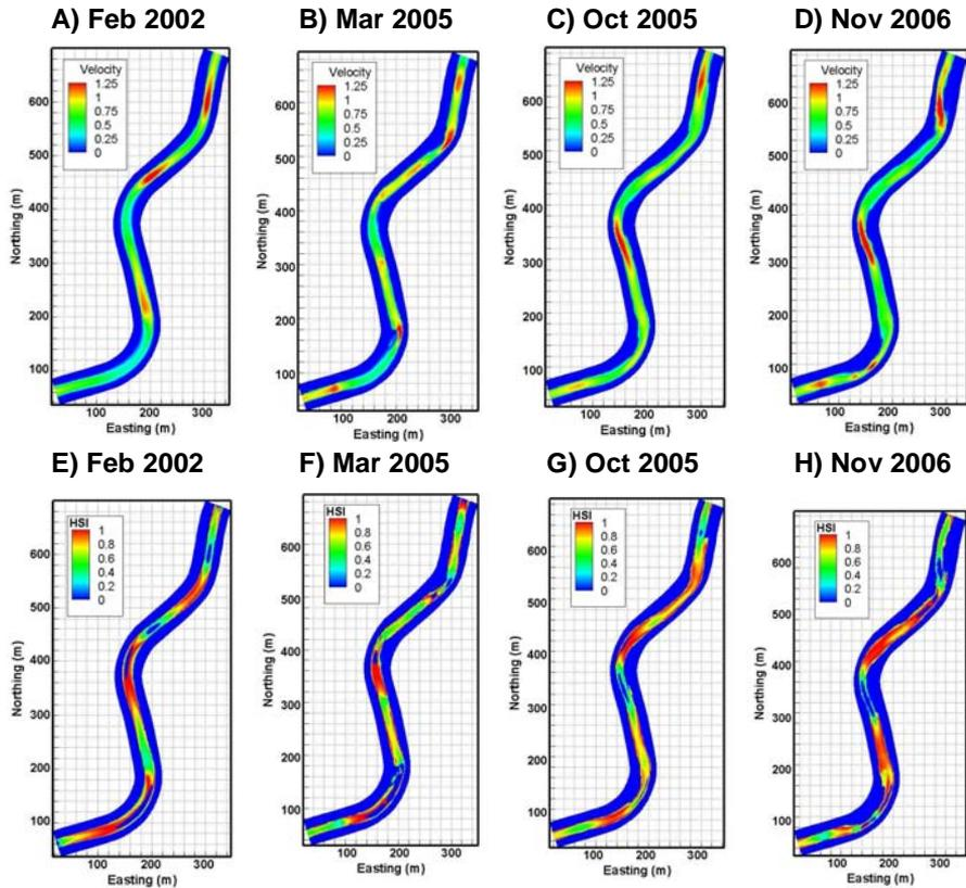
**Figure 3.** Model simulations of velocity (A-D) and the Habitat Suitability Index (E-H) for a discharge of  $6.4 \text{ m}^3/\text{s}$ .
