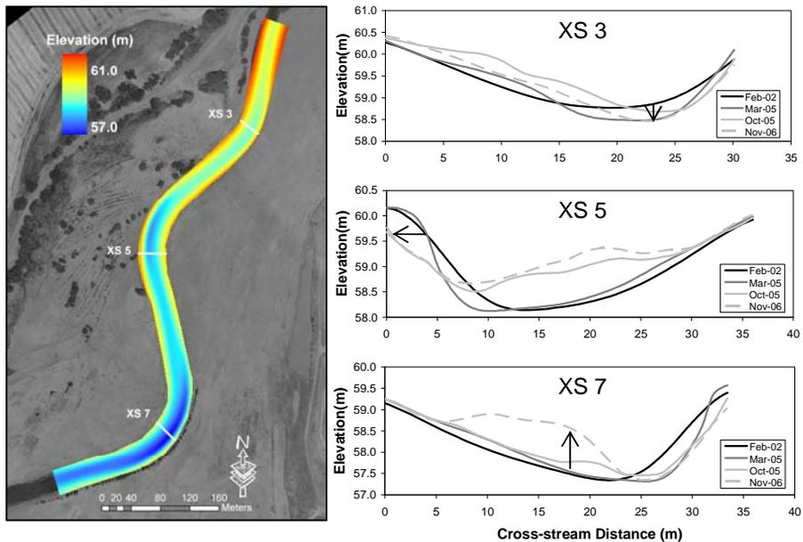
**Figure 2.** Cross-sectional change, illustrating trends in pool scour (XS 3), bank erosion (XS 5) and bar growth (XS 7).
